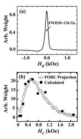
FIG. 3. Projection of the FORC distribution  $\rho$  of the 52 nm nanodots onto (a) the  $H_B$  axis, showing weak dipolar interactions; and (b) the  $H_C$  axis (open circles), showing a coercivity distribution that agrees with a calculation based on measured size distribution (solid circles).
